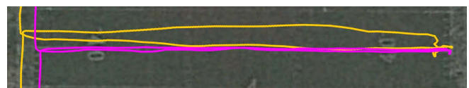
Figure 8: Localization comparison of the absolute \mu Blox solution (yellow) to the relative APT solution (pink)
